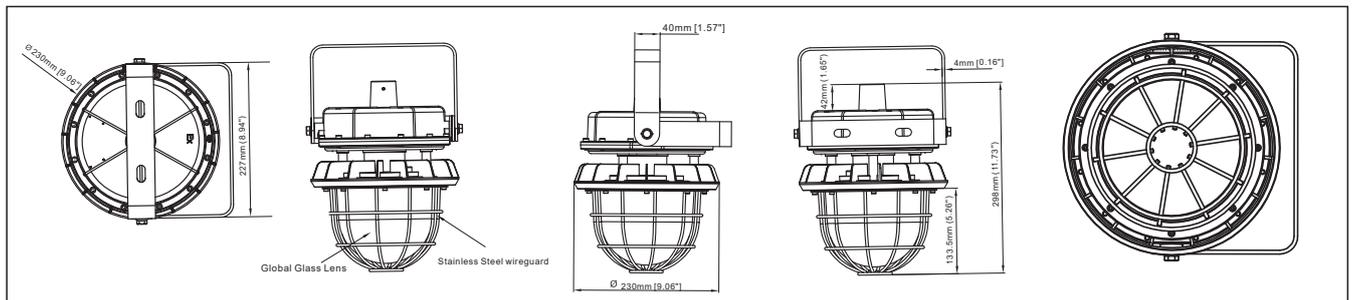
This structure type with bracket, global glass lens and wireguard to generate 180° light distribution.
