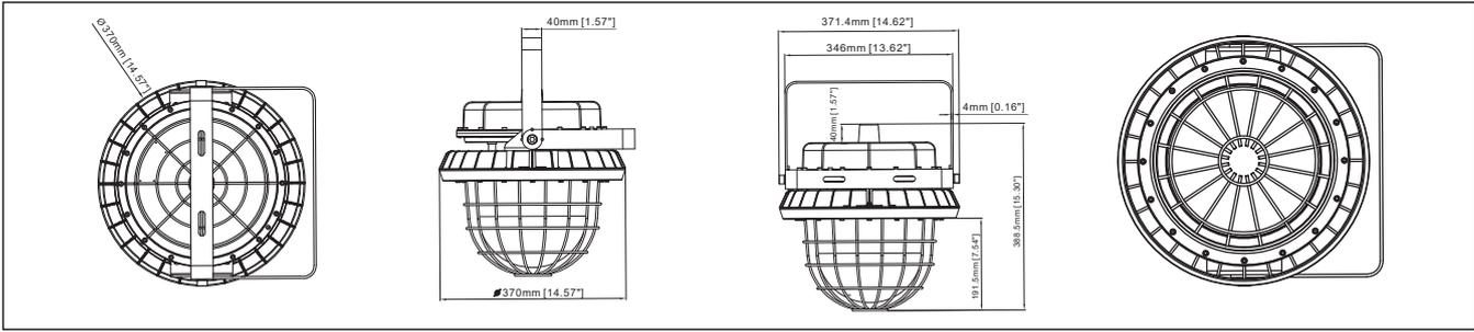
This structure type with bracket, global glass lens and wireguard to generate 180° light distribution. We also can put corn bulb in the global glass lens to make this beam angle up to 360°.
