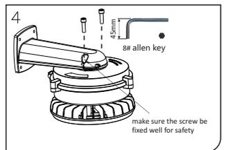
4. Tighten 2x screws to avoid the lamp loosened.
