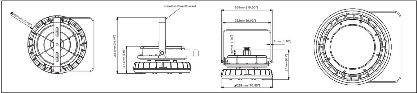
This structure type with bracket, flat glass and optics lens to generate 40°, 60°, 90° and 120° light distribution.
